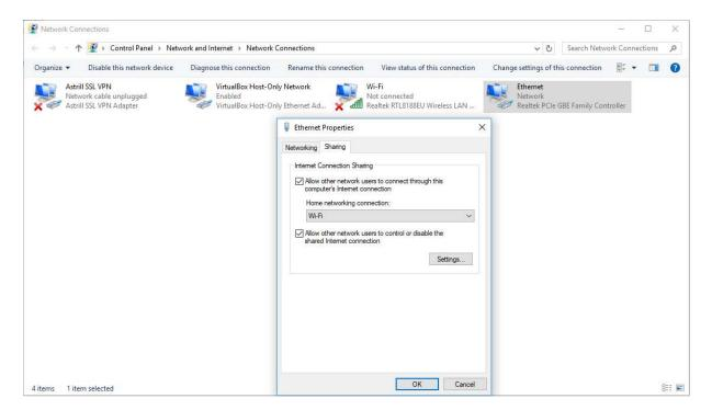
[Optional: set static IP address for the Ethernet connection]
