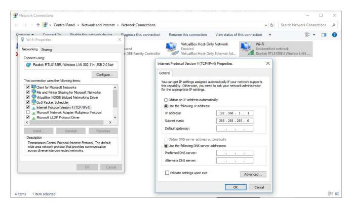
Connect to Raspberry Pi (Access Point). The AP name is "Monocilindro", the password is "raspberry".
