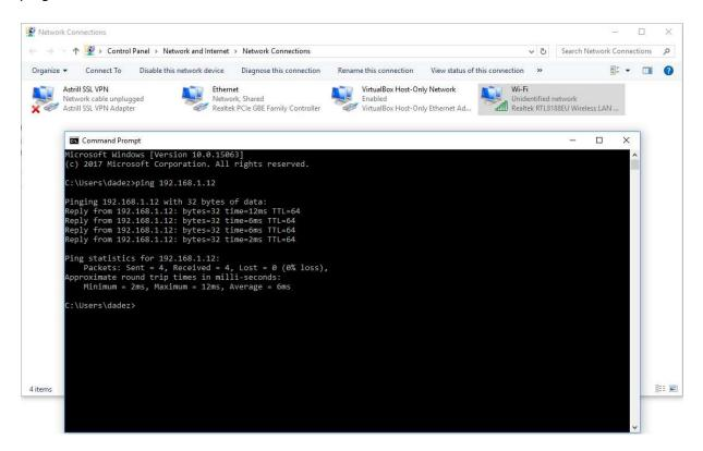
Connect to Raspberry Pi using VNC Viewer. From Raspberry Pi (192.168.1.12), check "ifconfig" and ping "google.com". If you get a reply, it means that the configuration is working properly.
