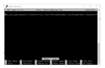
Save, exit, and restart. At next Power On, you Raspberry will be writeable again. You can double check it by typing "df" command. "overlay" should not be shown. Now, for example, you can install new programs and run updates (sudo apt-qet update).
