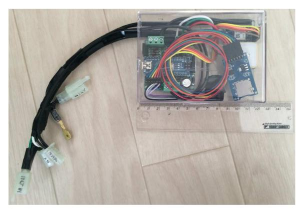
The following picture shows the electrical wiring on a Fuelino Proto3. The schematic is general: of course it is valid for a Honda CBR125R, but it may be extended also to other motorcycles equipped with Electronic Fuel Injection, such as: Kawasaki Ninja 250R, Kawasaki D-Tracker 250, Honda CBR250R, Honda CRF250L, Yamaha R125, Yamaha R25, Aprilia RS4 125, KTM Duke 125, KTM Duke 250, KTM Duke 390, and so on.
