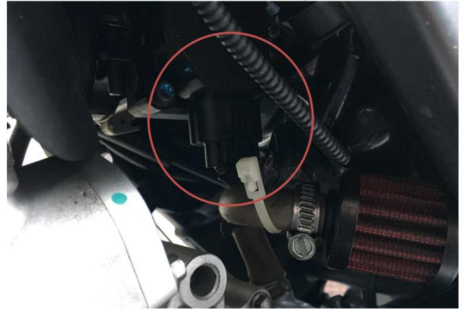
For the Lambda sensor (O2 sensor), it is quite the same as for the throttle signal: it is necessary to "sniff" the signal coming out from the Lambda sensor. You can just cut the lambda sensor wire, connect a sniffing cable, and crimp again, as shown below.
