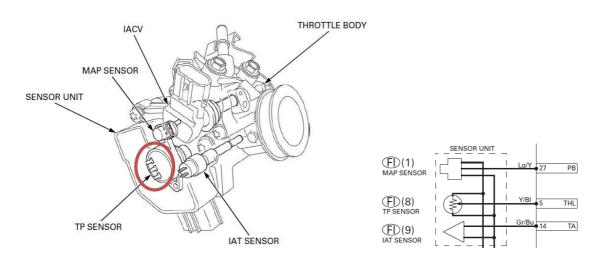
Below, a practical example is shown: just cut the wire, connect the "sniffing" cable, and connect again.
