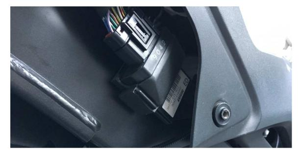
Or you can intervene as below, which is the same as visible in the theoretical scheme in the previous page. There are 2 cables: one is from the original Keihin ECU (12V, INJ\_IN), and one is Fuelino output (12V, INJ\_OUT). Both cables are going under the seat, so they can be easily connected to Fuelino. To summarize, there are 2 cables, each one with 2 pins, going under the seat.
