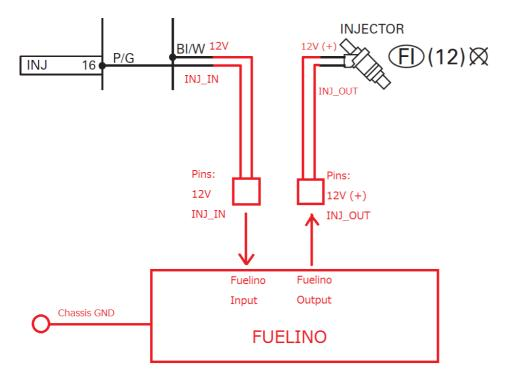
For this modification, you can intervene directly on the Keihin ECU connector cables.
