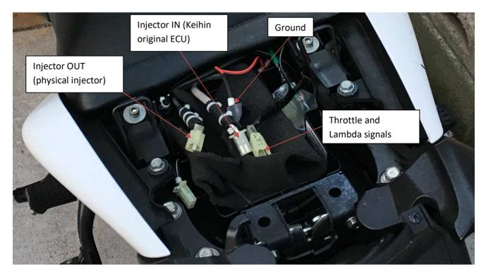
The picture below shows an example of complete Fuelino Proto3 system. It has the following connectors:
