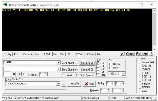
The following picture shows the message received from Fuelino, when it is fed with 10Hz, 5% duty cycle injection input pulses, which means that the distance between injections is 100 milliseconds, and the injection time is 5 milliseconds.
