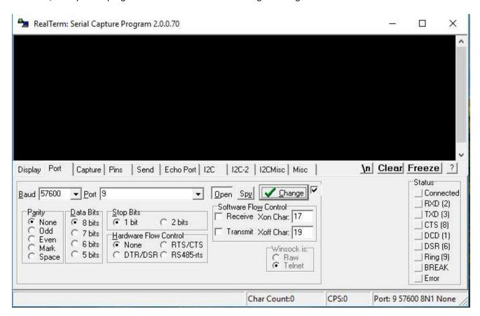
Each service command sent from service tool (PC) to the Fuelino, via USB cable (Serial communication), is composed by 8 ASCII characters (1 ASCII character = 1 byte) plus a final "line feed" or "line return" ASCII character.
