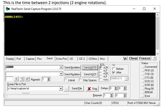
"d001" replies with "628" (about 2500us). This is the input injection time.
